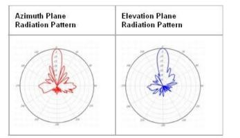
Cisco AIR-ANT3338 21dBi Parabolic Dish Azimuth 3dB BW =12° Elevation 3dB BW =12°
